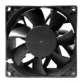
Frame: Thermoplastic PBT UL 94V-0 Impeller: Thermoplastic PBT 94V-0 Ambient Temperature Range: -10°C ~ +70°C Bearing: Ball or Sleeve Termination: Terminals or Lead wire Weight: 202 g
