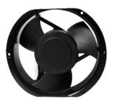
Frame: Aluminum Impeller: Thermoplastic PBT 94V-0 Ambient Temperature Range: -10°C ~ +70°C Bearing: Ball Termination: Terminals or Lead wire Weight: 655 g
